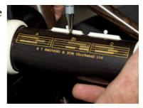
Complete tuning by then positioning slide (3) to harmonize with slide (1)
