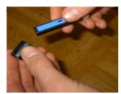
2. Remove the damaged blade and discard
